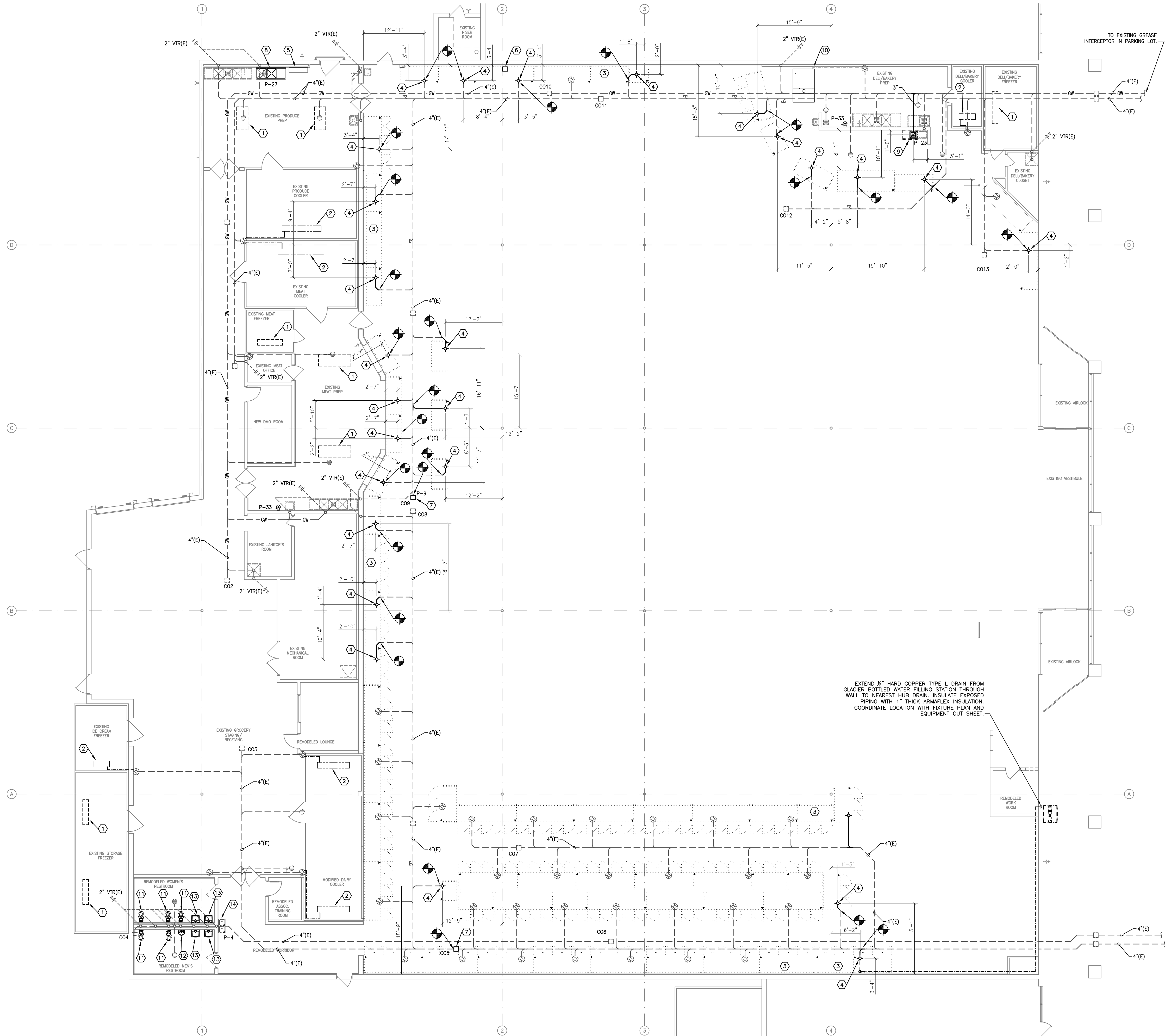
1 SANITARY SEWER AND DRAIN PLAN P1.01 SCALE: 3/32" = 1'-0"
